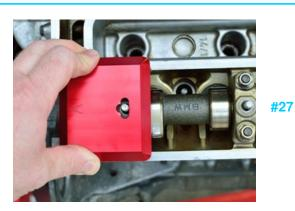
Once the block is seated flat against head surface it should look like this, with the stud centered in the T-slot.
