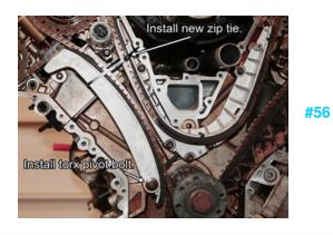
Install tensioner guide rail bolt, and torque to 22Nm - 16ft/lbs.
