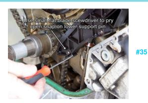
After removing the hex bolts, use a small flat blade screwdriver to pry the clip at the bottom of the guide, then slide the guide from the retaining pins.
