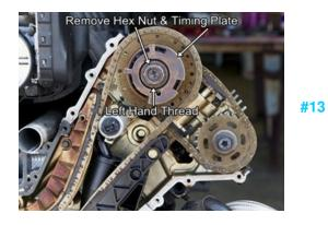
Remove the hex nut and timing plate on bank 5-8 with a 24mm socket or wrench.
