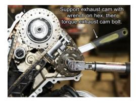
You will now torque the exhaust cam sprocket bolts. Make sure to support the camshafts with a wrench on the hex section of the cams while torquing. Do not apply the tightening torque against the cam lock blocks.
