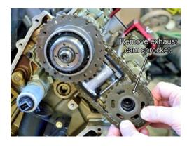
With the tensioner compressed, remove exhaust cam sprocket as shown.
