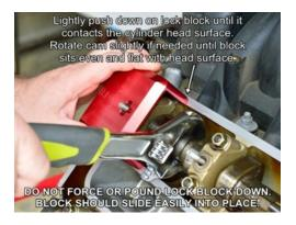
Lightly push down on block until it seats against cylinder head surface. Rock the camshaft a little back or forth if necessary until block sits flat to head.
