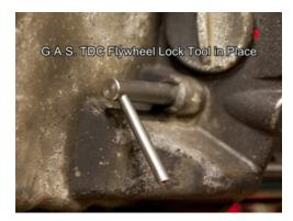
Make sure that you have set cylinder number one piston at TDC (Top Dead Center) of the compression stroke, and that you have installed the TDC flywheel lock pin that comes with the kit.
