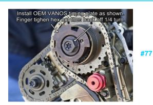
Install the VANOS timing plate and hex nut onto bank 1-4 intake cam.
