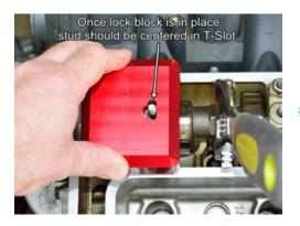
Once the block is seated flat against head surface it should look like this, with the stud centered in the T-slot.
