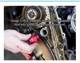
Install the German Auto Solutions VANOS alignment threaded tool into the two VANOS solenoid locations.
