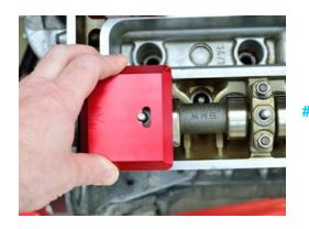
Now slide the block toward the front of the engine until the stud stops against the end of the T-slot. This fully engages the block over the square boss on the end of the camshaft.
