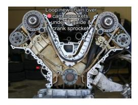
Next loop your new primary timing chain over the intake cam sprockets, under the U-shaped guide, and under the crankshaft sprocket.
