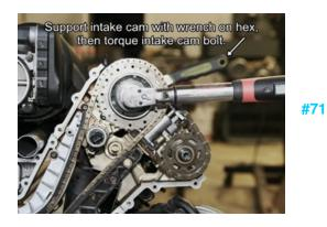
You will now torque the intake cam sprocket bolts. Make sure to support the camshafts with a wrench on the hex section of the cams while torquing. Do not apply the tightening torque against the cam lock blocks.
