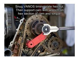
With VANOS timing tool engaged with timing plate, snug the timing plate hex nut, then torque to 40Nm - 30ft/lbs.
