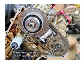
You will now remove the exhaust sprocket on bank 5-8.
