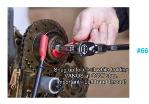
While holding CCW tension on the wrench and verifying continuity, snug the intake cam sprocket bolt, but do not torque yet.
