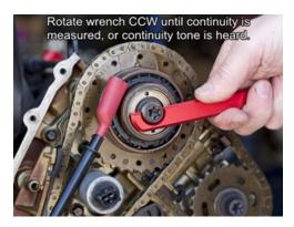
The VANOS unit will have oil remaining inside and may be difficult to turn until the oil is purged. I like to rotate the unit back and forth a few times until I can feel the oil has been purged from the unit. This is absolutely necessary if you are not using a multimeter for this procedure.
