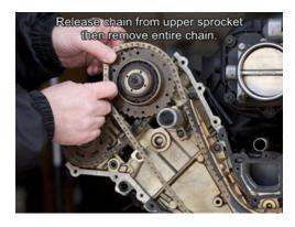
Release the primary chain from bank 1-4 intake cam sprocket, then remove entire chain.
