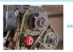
Install the VANOS timing plate and hex nut onto bank 5-8 intake cam.
