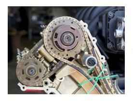
We will now start the disassembly of the primary timing chain guides.
