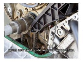
Slide your new stationary chain guide over the two retaining pins until guide snaps into place.
