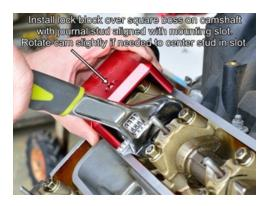
You will now install the camshaft lock blocks stariting with cylinder bank 5-8.
