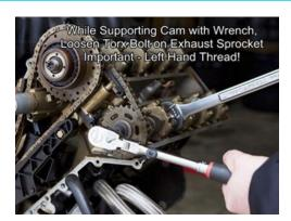
While supporting the exhaust camshaft with a 27mm or large adjustable wrench, loosen the torx bolt on the exhaust cam sprocket of bank 5-8.
