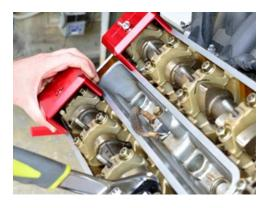
We will now repeat the procedure on the exhaust camshaft. Exhaust cam pictures lack the text of the intake cam pictures. The procedure is identical.
