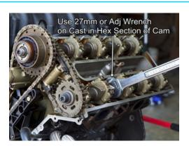
In the following steps you will need to support the camshaft with a 27mm open end or adjustable wrench placed over the cast hex shaped portion of the camshaft as shown.
