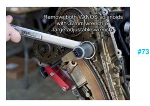
Remove the VANOS solenoids on both cylinder banks using a 32 mm wrench or a large adjustable wrench.
