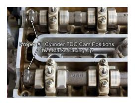
With the crankshaft locked at #1 cylinder TDC position, your bank 1-4 and 5-8 cam markings should be facing up. If the markings are facing down, rotate the crankshaft one full revolution and reinstall the TDC lock pin. See step #70 for an easy way to help find TDC again if you need to rotate the crank.
