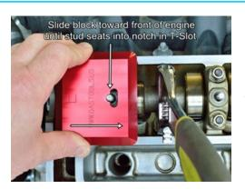
Now slide the block toward the front of the engine until the stud stops against the end of the T-slot. This fully engages the block over the square boss on the end of the camshaft.
