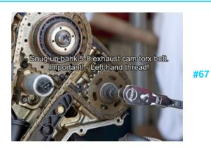
After you have snugged, but not torqued the intake sprocket bolt, snug but do not torque the exhaust sprocket bolt.
