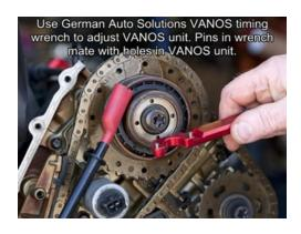
Using your German Auto Solutions VANOS adjusting wrench, you will be rotating the inner section of the VANOS unit counterclockwise until the multimeter reads continuity or an audible tone is heard.
