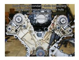
Compress your new secondary chain tensioners, then insert the locking clips from your tool kit to keep them compressed.
