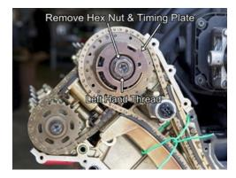
Start by removing the hex nut and VANOS timing plate on cylinder bank 1-4 with a 24mm socket or wrench.
