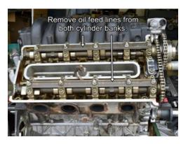
Remove the 10 hex nuts securing the cam journal oil feed lines, then remove the oil feed lines from both cylinder banks.
