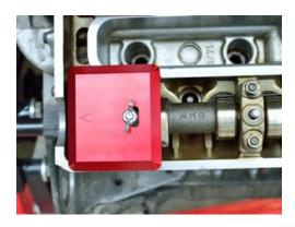
While keeping downward pressure on the lock block, install the provided 6mm wing nut and finger tighten.
