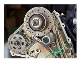
Bank 1-4 nut and timing plate removed.
