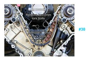
Remove the two 7mm torx bolts, and the three 6mm torx bolts securing the U-shaped guide using an E10 Torx socket.
