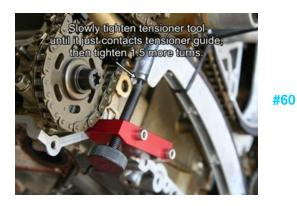
Now tighten tensioner tool thumbscrew until tensioner pin just contacts guide rail, then tighten tensioner tool 2 more turns to set proper chain tension.
