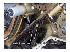
Now install the two hex bolts at the top of the guide. Snug the two bolts, then torque to 10Nm - 7.5ft/lbs.
