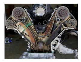
This should be your starting point, with valve cover, accessories and all timing covers removed, and the engine set at #1 cylinder TDC compression stroke.
