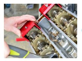
Lightly push down on the block until it seats against cylinder head surface. Rock camshaft a little back or forth if necessary until block sits flat to the head.
