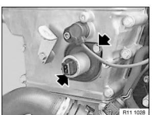
Insert screws on sealing flange and tighten down. Assemble engine.
