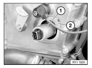
Clean solenoid valve (1) and sealing face (2).
