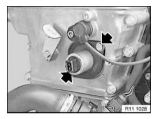
Release screws on sealing flange.
