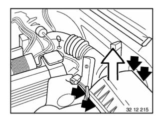
Remove upper section of suction filter housing style with mass air flow sensor.
