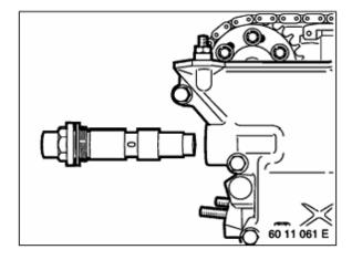
Remove screw connection and piston for chain tensioner.
