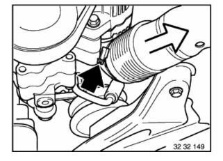
Remove brake air duct, left and right. Release retainer for pressure line from engine support.
