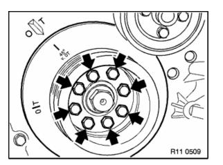
Release screws and remove vibration damper.
