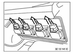
Disconnect plug connections on ignition coils.
