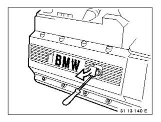
Remove sealing caps on covers of ignition coils.
