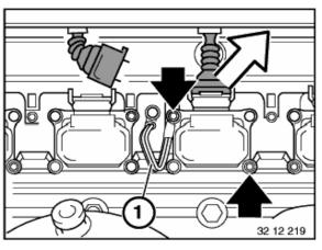
Release screw connections on ignition coils. Remove ignition coils.
