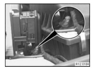
Unscrew screw. Remove complete filter housing.
