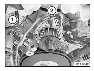
Only release bolts (2) on water pump bracket.
