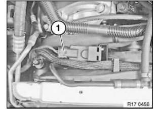
Unlock plug (1) on AUC sensor and disconnect.
